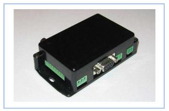
Can change the serial port speed according to IEC1107 Mod C. So it can attune itself to the meter speed while reading data and provides a fast reading.
